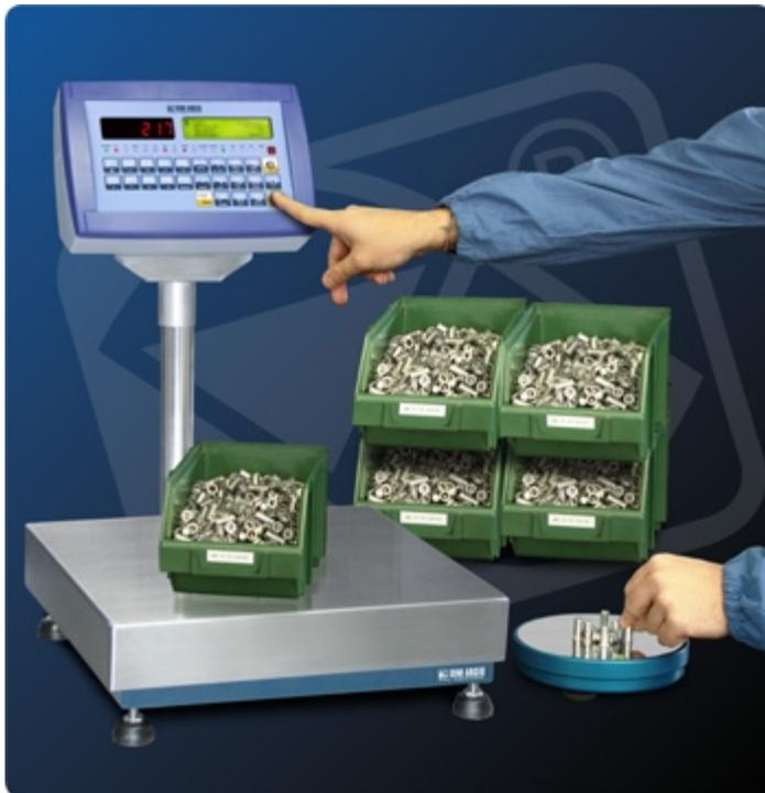
Solution for mono or multi scale, pieces or quantity (litres, metres, Newton etc) counting systems, suitable for the inventory checking and the quick and precise counting of high quantities of pieces. It is possible to create your own custom-made solution, by choosing the weight indicator and the most suitable platform among those listed in the tables below. The system can also be enriched and enhanced through the many available options.
